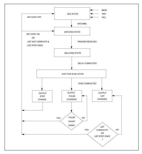
Figure 4-2. Model of Output Triggers
