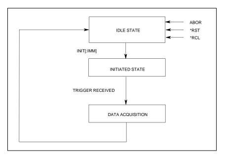
Figure 4-3. Model of Measurement Triggers
