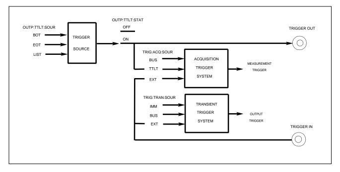
Figure 4-6. BNC Connector Trigger Model
